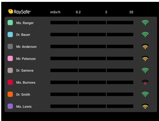
Figure 10. The Real-time View in Service mode . The signal strength for each connected dosimeter is indicated to the right.
