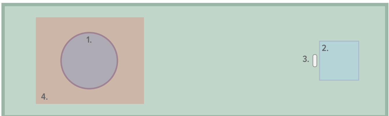
Figure 18. Performance verification arrangement. 1. Patient phantom. 2. Staff phantom. 3. Dosimeter. 4. X-ray field.
