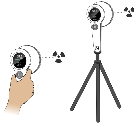
Figure 3. Position with the sensor area facing the radiation source.
