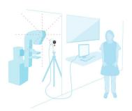
Tube leakage is the radiation emitted from the machine outside the primary beam. All X-ray tubes have some radiation leakage. Measurements are made around the tube housing, at positions where personnel typically stand during a surgery. From tube leakage measurements, calculations are made to estimate an operator's body radiation dose, for a single exposure or over an extended period.
