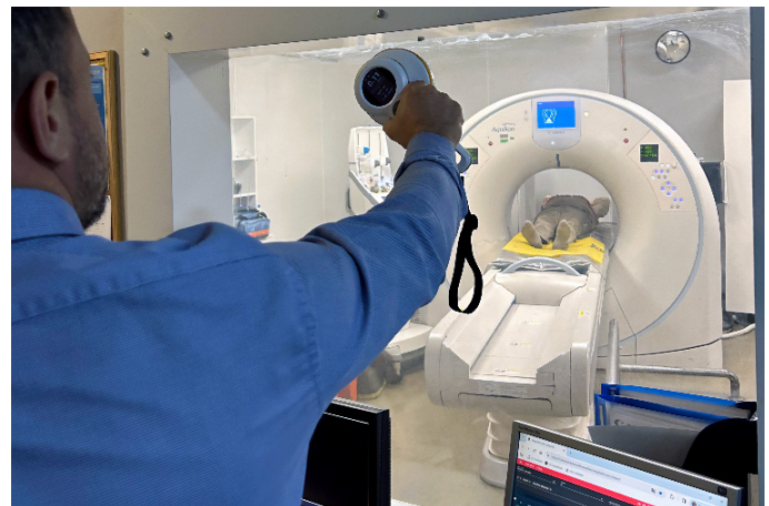
The RaySafe 452 is calibrated with traceability to PTB, an internationally recognized primary standard equivalent to NIST according to mutual recognition agreements used for international metrology. Both standards are traceable to the SI.
