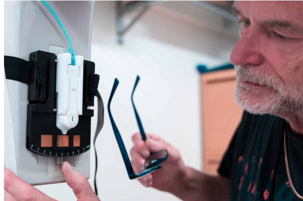
The RaySafe X2 Panoramic Holder is a convenient tool to help position the sensor in the center of the narrow radiation field.
