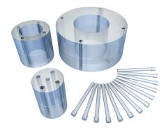
dose to a patient during a CT scan procedure. Measurements are done with a pencil shaped ionization chamber together with a phantom simulating a patient.
