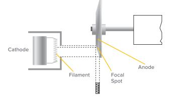
X-ray is produced inside a vacuum container of glass or metal. The reason why it has vacuum inside is that electrons cannot be accelerated in air.
