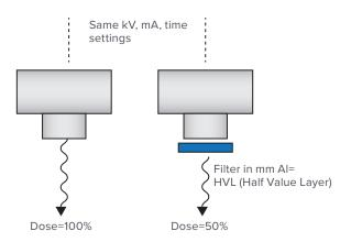
More shielding will affect the HVL. A low HVL means bigger share of low energy photons compared to a high HVL. And a change in HVL means a change in beam quality, which affects the X-ray image quality.
