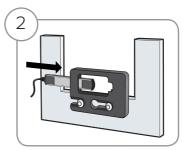
Insert the RaySafe Xi R/F detector into the radiography holder.
