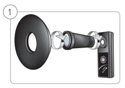
Mount the RaySafe Gx adapter to the RaySafe light detector according to the illustration.
