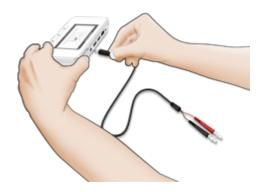
Connect the mAs cable to the base unit and to the generator.
