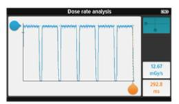
Slide the handles to view, for example, the peak dose rate of a pulse.
