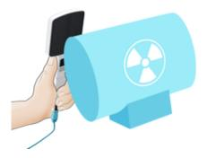
Position the sensor with the dark side towards the radiation source.
