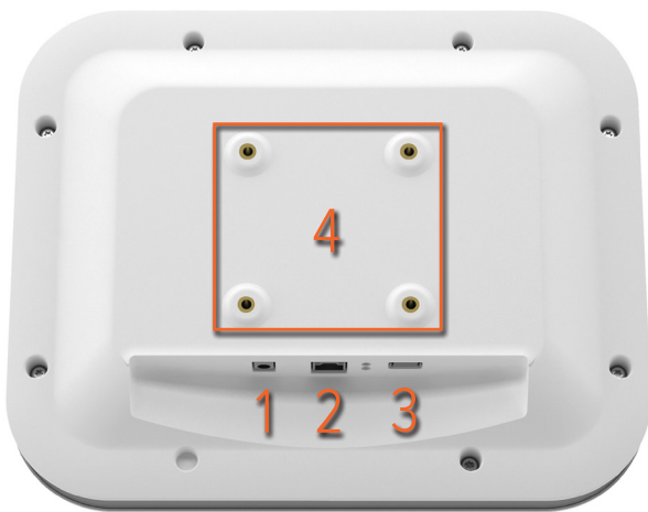
Figure 6. Interfaces (back side of the Real-time Display): 1: 12 V DC, 2: Ethernet, 3: USB, 4: VESA 75
