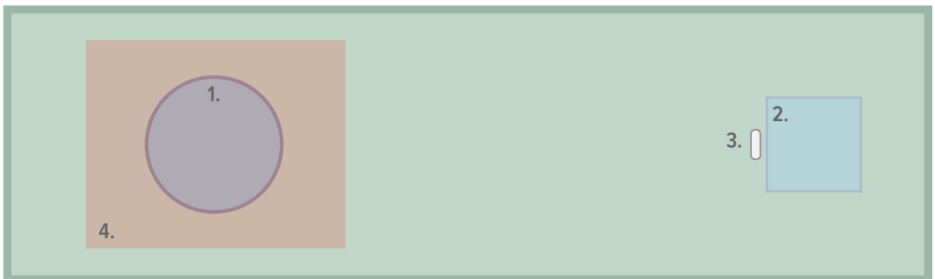
Figure 19. Performance verification arrangement. 1. Patient phantom. 2. Staff phantom. 3. Dosimeter. 4. X-ray field.
