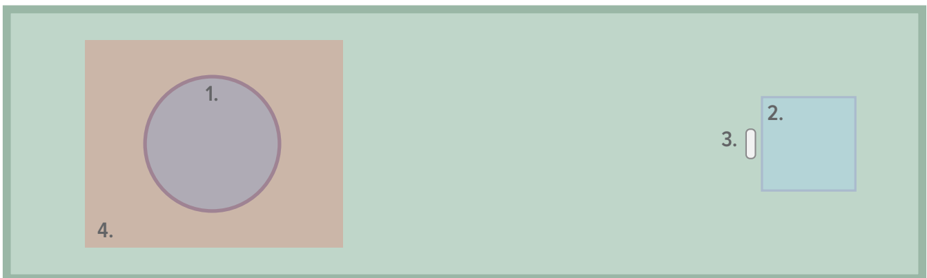
Figure 23. Performance verification arrangement. 1. Patient phantom. 2. Staff phantom. 3. Dosimeter. 4. X-ray field.
