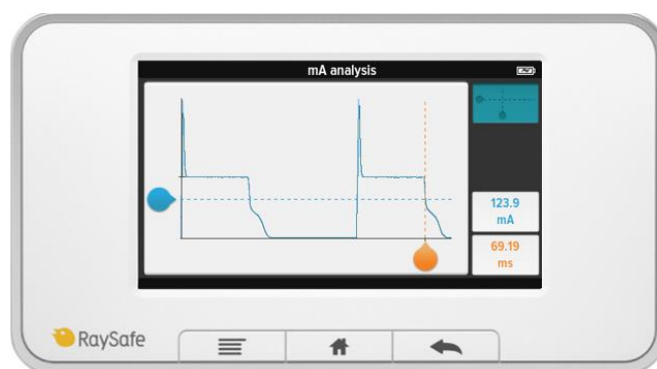
Figure 2: Illustration of an mA avg reading for a pulsed exposure. The dashed blue line shows the resulting value of 123.9 mA .
