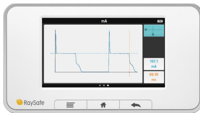
Figure 1: Illustration of an mA reading for a pulsed exposure. The dashed blue line shows the resulting reading of 197.1 mA .
