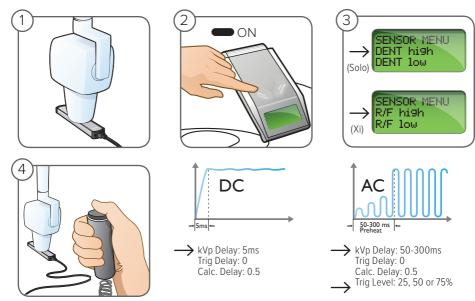
Note: the Set kVp delay or trig level depending on type of machine and waveform.
