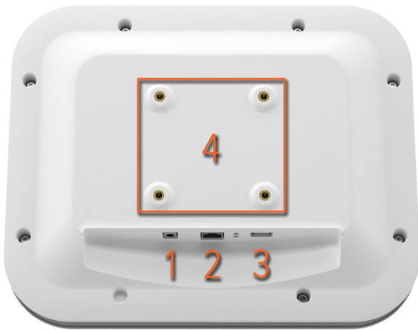
Figure 5. Interfaces (back side of the Real-time Display): 1: 12 V DC, 2: Ethernet, 3: USB, 4: VESA 75
